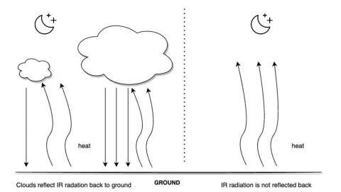
Lots of factors affect the actual sky temperature. Your geographical latitude, the ambient temperature and conditions in troposphere will shift the sky temperature so a correction model is automatically applied by the Uranus device.
