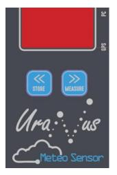
Keep pressing [>>] (Measure) button for 2 seconds to trigger a Sky Quality measurement. Remember to point the device towards the area of the sky you would like to acquire a light measurement.
